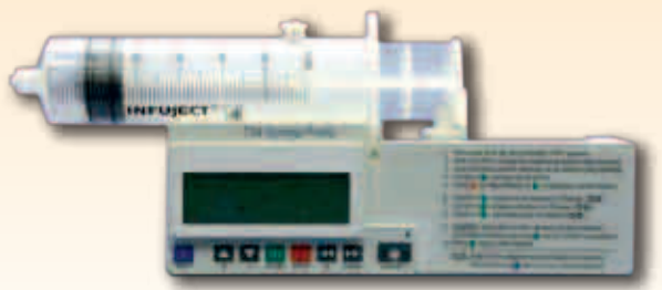
Syringe driver with motor driven linear actuator
