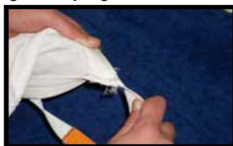
Frayed loop attachment: Unsafe to use
