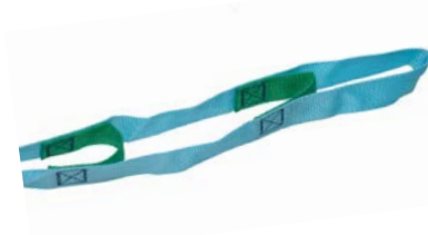
Intact loop attachments: safe to use
