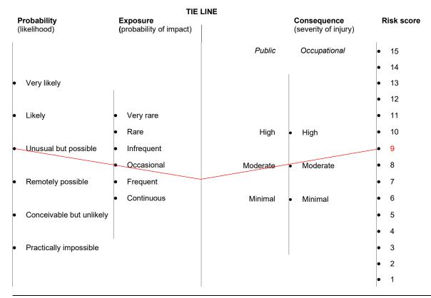
The risk score nomogram used to determine the relative safety risk for each parameter relevant to an ionising radiation practice:
