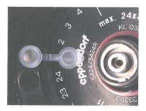
Figure 2: Placement of Eppendorf tubes in centrifuge
