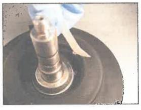
Removing plastic debris with tape.
