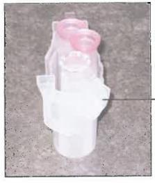
1.5 ml microcentrifuge tube lid is in the wrong slot of the rotor adapter
