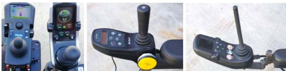
Figure 3: Example controls with different joystick handles, switches, levers, dials and buttons.
