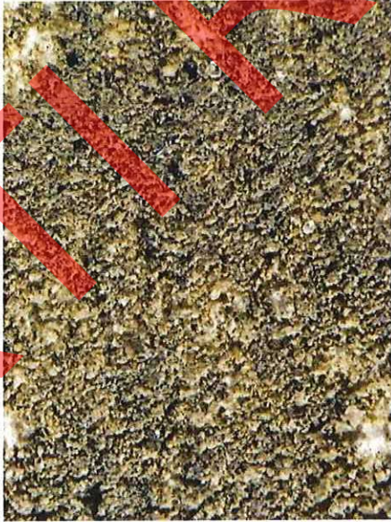
StMPM1. , CV-DSI-0417, UQMP # 14907. Very small dark brown to gold coloured particles with a number of black angular particulates, typical of coal noted and dispersed throughout the deposit.
