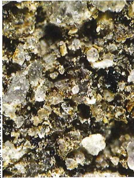
StMPM1. , CV-DSI-0417, UQMP # 14907. Very small dark brown to gold coloured particles with a number of black angular particulates, typical of coal noted and dispersed throughout the deposit.
