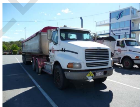
Figure 9a Covered and placarded vehicles carrying zircon mags – note front and rear signs
