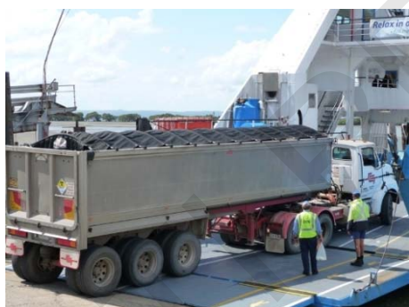
Figure 9a Covered and placarded vehicles carrying zircon mags – note front and rear signs
