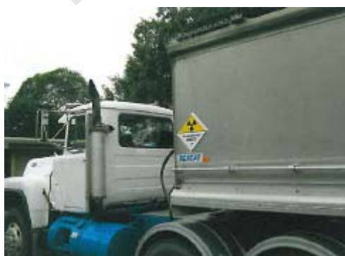
Figure 9b Modification to allow placarding on sides of vehicle
