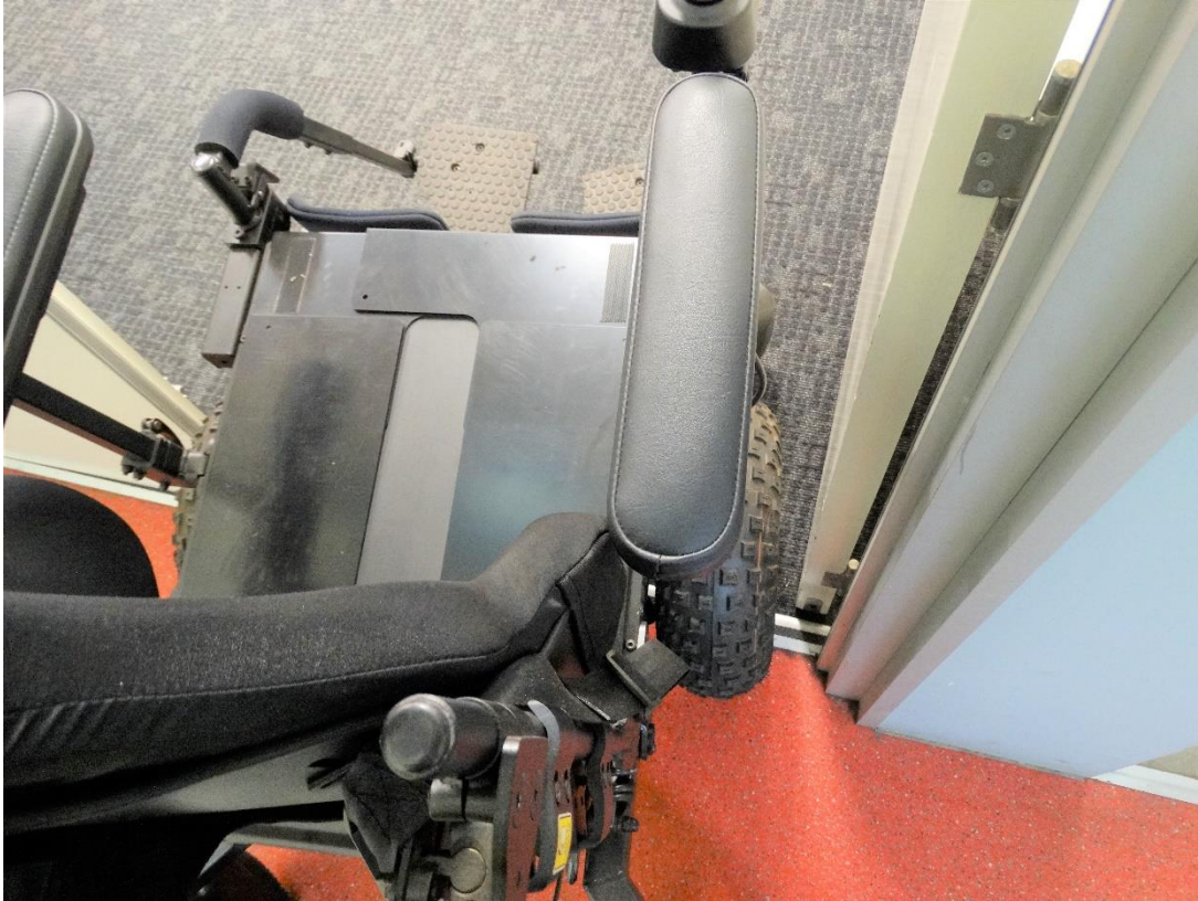
Power wheelchair overall width 740mm passing through a doorway clear open 803mm
